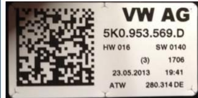
Label on slip ring controller
